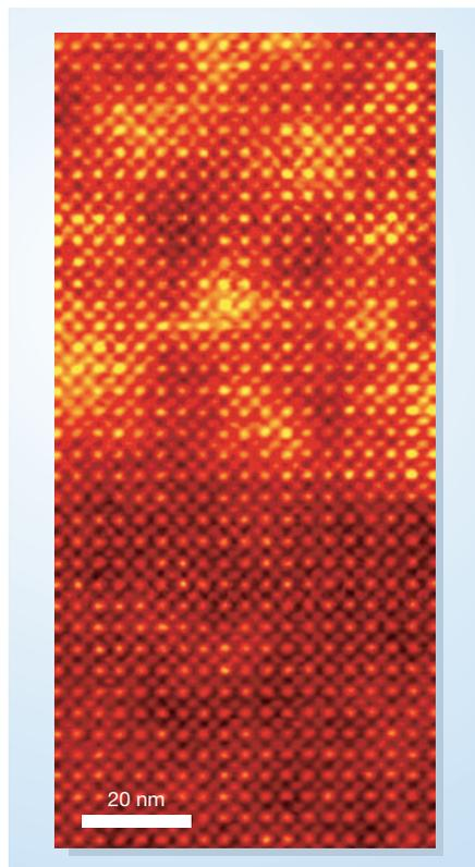
**Figure 2** What a difference a layer makes. The abrupt junction between layers of SrTiO<sub>3</sub> (bottom) and SrTiO<sub>3- $\delta$</sub>  (top) is clear in this image created by Muller *et al.*<sup>3</sup> using a scanning transmission electron microscope. Each bright-orange blob is a cluster of oxygen vacancies.
